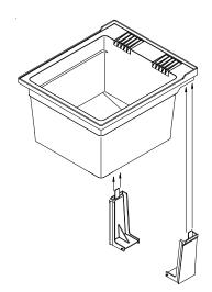
Attach the filler plates to the back of the tub as shown. The tongue on top of the filler plate should fit into the groove under the backside of the tub. The attachment pins on the bottom of the filler plates will align with the holes in the tub. Note that there is a left and right filler plate. If they are not used on the correct side the pins will not align with the holes. The filler plate may need to be tapped with a hammer to push the pin into the hole completely.
