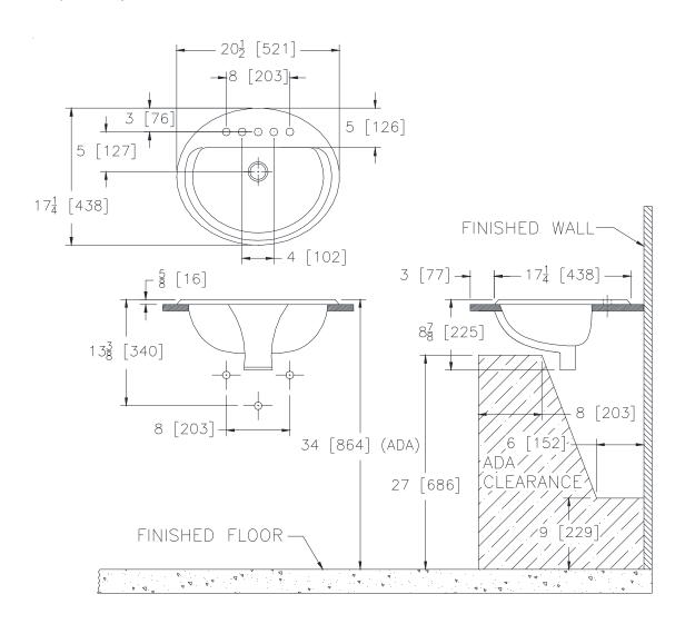
Fixture dimensions meet ANSI/ASME standard A112.19.2 and CAN/CSA B45 requirements.
