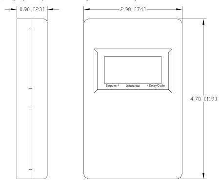
**Engineering Specification:** Zurn One-Stage Setpoint Control for heating and cooling. This is a 24VAC microprocessor-based control. This unit will maintain a fixed setpoint by cycling a heating or cooling device. This controller features a wide setpoint range, adjustable differential, and time delay. Unit has an easy to read LCD window. Output is 24VAC, 8 amp relay. Includes one QHUS universal 10K ohm sensor.
