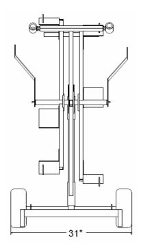
**Engineering Specification:** Zurn QDISP Tubing Uncoiler. Holds and dispenses two Zurn PEX $^{\circledR}$  coils. Use with stretch wrapped or tapped coils. Adjustable discharge arm.
