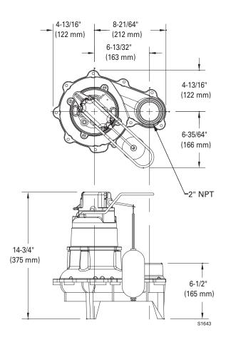
NOTE: The sizing of effluent systems normally requires variable level float(s) controls and properly sized basins to achieve required pumping cycles or dosing timers with nonautomatic pumps.
