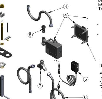
A Maximum of (8) ChekPoint Faucets can be Hardwire Connected and Powered by EC-HARDWIRE ChekPoint Hardwire AC Transformer. (Sold Separately) –
