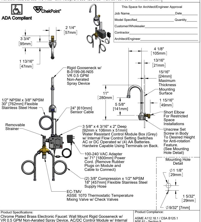
Flow Control Setting Switches, Thermostatic Temperature Control Mixing Valve w/ Check Valves, 18" Flexible Stainless Steel Supply Hoses
