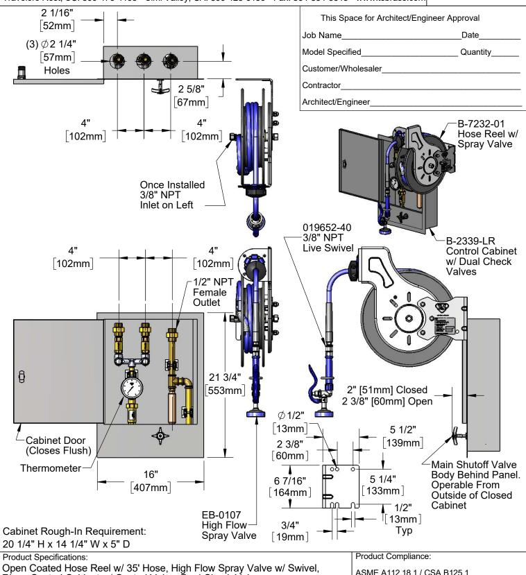
Rinse Control Cabinet w/ Control Valve, Dual Check Valves,
