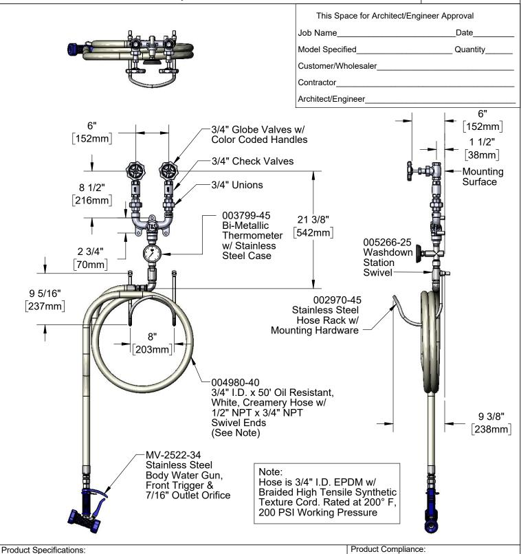
Hot & Cold Water Washdown Station w/ Thermometer, Mixing Valve w/ 3/4" NPT Inlets, 50' Creamery Hose w/ Water Gun & Hose Rack
