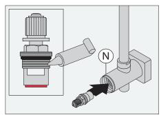
**Installation Tip:** Back off cartridge slightly to ensure proper handle alignment if necessary.
