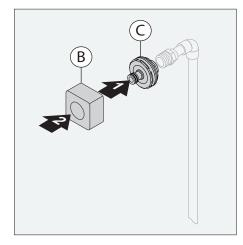
**Note:** Apply plumber tape to water connector (C).
