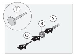
**Note:** For dry wall 1/2" thick or less, insert anchor tool (T) into toggle anchor (S) to secure behind wall prior to installing trim.
