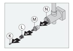
Apply removable thread lock to the threading of replacement cartridge. Install replacement cartridge into diverter body (N) at 50 in•lb.
