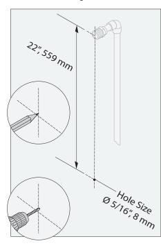
2) Insert toggle anchor (S) into 5/16" hole. Locate mounting ring (R) over toggle anchor (S) and secure to wall with mounting screw (Q).
