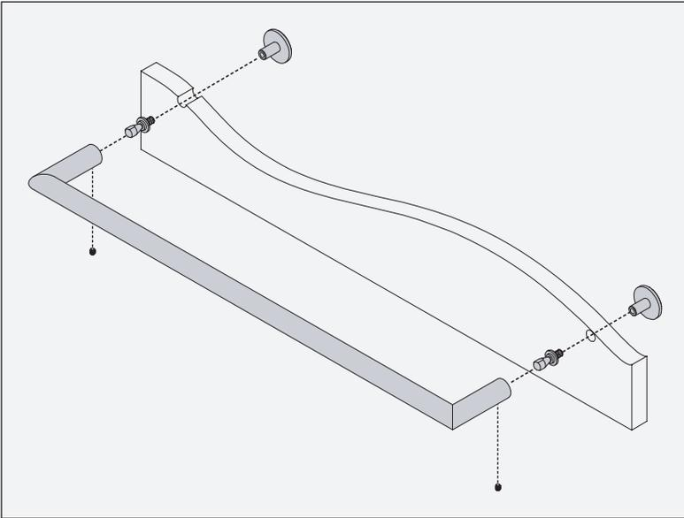
**Note:** Apply a bead of silicone around the perimeter of trim installed flush to finished wall.
