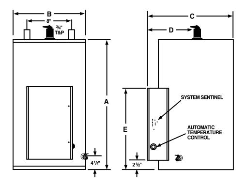
• System Sentinel: All models employ a diagnostic panel utilizing light emitting diodes (L.E.D.), corresponding to the number and location of each heating element. L.E.D.'s are energized when the electric elements are operating. An unlit L.E.D. pinpoints the exact location of a non-functioning element, making element operation diagnosis simple and positive.
