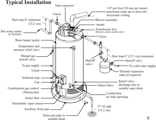
A new combination temperature and pressure relief valve, complying with the Standard for Relief Valves for Hot Water Supply Systems, ANSI Z21.22/CSA 4.4, is factory installed and must remain in the opening provided and marked for the purpose on the water heater. No valve of any type should be installed between the relief valve and the tank.
