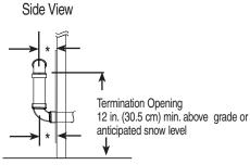
\* Clearance is equal and parallel to wall 4 in (10 cm) for 2 in (5.1 cm) pipe 5.5 in (14 cm) for 3 in (7.6 cm) pipe
