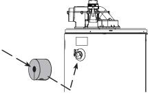
Typical Side Connect T & P Arrangement.
