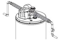
Typical horizontal piping arrangement
