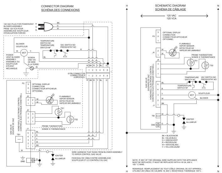
120V 50/60 Hz Less Than 5 Amps 120V 50/60 Hz, Moins de 5 A
