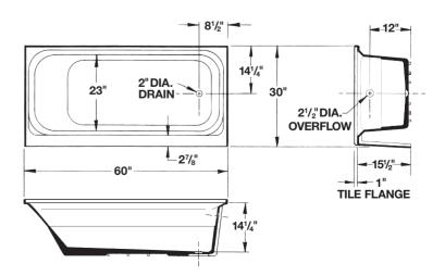
General: Furnish and install as shown on plans, E.L. Mustee & Sons, Inc. TOPAZ™ Fiberglass Bathtub 30" x 60" right or left-handed Model: Construction shall be molded, reinforced fiberglass using matched metal molds under extreme heat and pressure. Shall meet ANSI Specification Z 124.1.2. Color: (White, Bone, Biscuit). Install in compliance with local codes.
