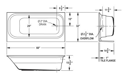
General: Furnish and install as shown on plans, TOPAZ® bathtub as manufactured by E.L. Mustee & Sons, Inc. Shall be a fiberglass 32" x 60": right hand or left hand Model \_\_\_\_\_\_. Construction shall be molded, reinforced fiberglass using matched metal molds under extreme heat and pressure. Shall meet ANSI Specification Z 124-2017. Color: \_\_\_\_\_\_ (White) Weight: 55 lbs. Install in compliance with local codes.
