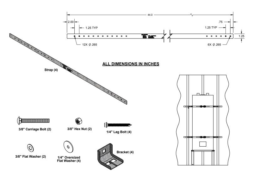
The HR-80-180 is a seismic/earthquake support system for water heaters up to 80 U.S. gallons in size. The system includes: (4) 44" Straps, (4) Brackets, (2) 3/8" Flat Washers, (2) 3/8" Carriage Bolts, (2) 3/8" Hex Nuts, (4) 1/4" Lag Bolts and (4) 1/4" Oversized Flat Washers.
