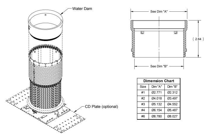
The HOLDRITE® Hydroflame Pro Series "Water Dam" attaches to the top of the Pro Series cast-in-place firestop sleeves and adds a 2" tall water dam barrier at the perimeter of the sleeve opening. Sizes are available to fit all Pro Series Sleeves, for all sizes of penetrants 1/2" thru 6" nominal size. See Riser Clamp load rating chart below. Thread sealant may be added to male threads prior to installation, if desired. UL-Listed accessory when used with HoldRite's Hydroflame Pro Series Sleeves.
