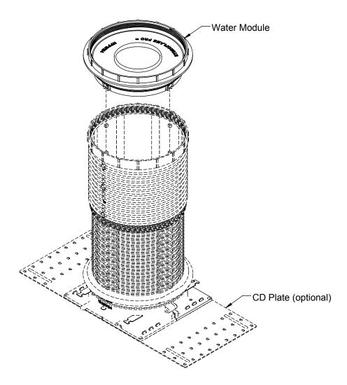
The HOLDRITE® Hydroflame Pro Series "Water Module" (#HFPWM1 - #HFPWM6) attaches to the top of the Pro Series Sleeves and provide a water, smoke and debris stop for 1/2" thru 6" piping. It is a UL Listed, W-Rated accessory that is cast into concrete or can be attached to Pro Series "Water Dam" fittings. Adds 1/2" to height of sleeve.
