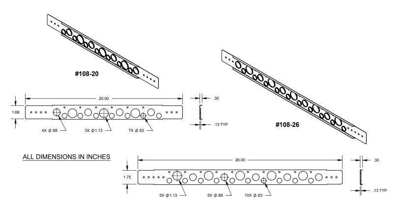
The HOLDRITE #108-20 and #108-26 are Copper-Bonded™ steel brackets with holes for 1/2" pipes on 2" centers, holes for 3/4" and 1" pipes on 4" centers. Featuring a rolled-edge for added strength, and extruded holes for easier soldering. The #108-20 & #108-26 are designed to positions copper water supplies for urinals, lavatories and other fixtures. When soldering, heat the pipe, not the bracket.
