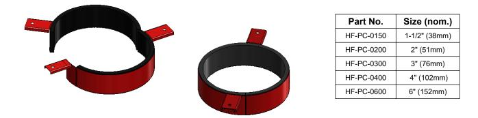
HydroFlame Pipe Collars are prefabricated for both open and closed through-penetration firestop systems using 1-1/2" (38mm) to 6" (152mm) plastic pipe. An easy interlocking tab assures fast and easy installation. The design of the collar greatly reduces the time and expense that is required to install competitive collars.
