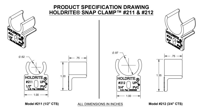
The HOLDRITE® #211 and #212 Snap Clamps™ are flame retardant and secure Copper, PEX and CPVC. Glueable when used with CPVC. Mounts to Stout™ or EZ-Strut™ brackets or directly to framing. Available for 1/2" and 3/4" tube sizes. (S) series clamps are 25/50 Flame Rated and non-glueable.
