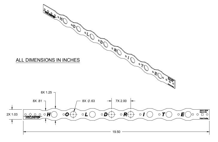
The HOLDRITE #100-18 is a Copper-Bonded™ steel bracket with 5/8" holes on 2" centers to support 1/2" copper tubing. The #100-18 positions copper water supplies for sinks, water closets, and other fixtures. When soldering, heat the pipe, not the bracket.
