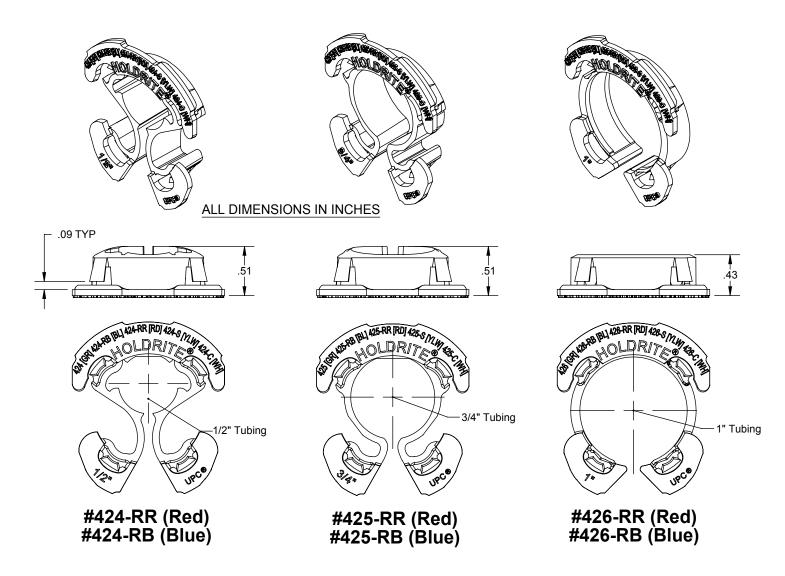
For used with 1-11/32" or 1-3/8" round cut-outs in 14 to 25 gage sheet metal. Ideal for isolation of Copper, PEX or CPVC tubing. Complies with UL94V-2 fire rating.
