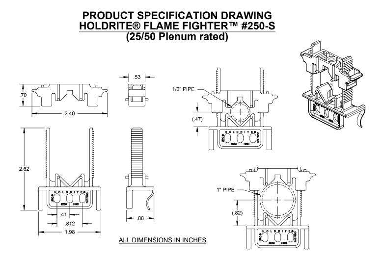
The HOLDRITE® Flame Fighter™ #250-S is a flame and smoke rated variable closure clamp compatible with Copper, PEX, CPVC tubing, conduit, etc. Supports up to 1" CTS tubing sizes. Material meets ASTM E-84 25/50 and UL94V-0 fire rating.
