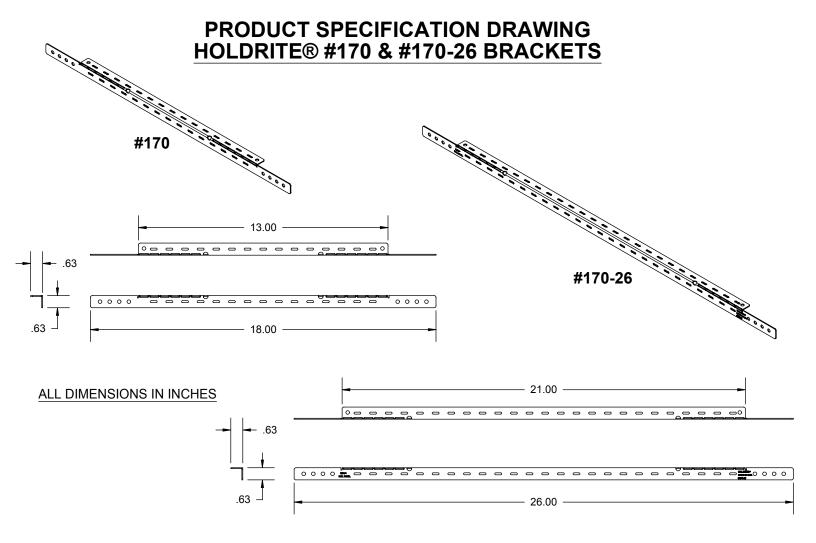
Versatile, galvanized steel brackets providing a platform for horizontal or vertical tube support. Also ideal for shower head, diverter, tub spout and sink applications. Use HOLDRITE #251 Rapid Clamp™, Pro Clamp™, Stout Clamp™ and other industry clamps. Perforated tear feature allows brackets to fit into narrow stud bays. Bendable end tabs allow brackets to be recessed into stud or joist bays.
