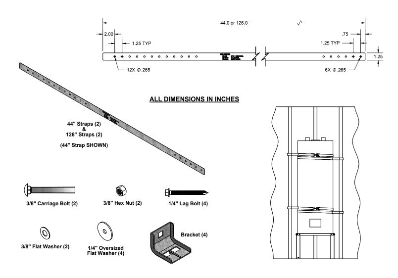
The HR-80-360 is a seismic/earthquake support system for water heaters up to 80 U.S. gallons in size. The system includes: (2) 44" Straps, (2) 126" Straps, (4) Brackets, (2) 3/8" Flat Washers, (2) 3/8" Carriage Bolts, (2) 3/8" Hex Nuts, (4) 1/4" Lag Bolts and (4) 1/4" Oversized Flat Washers.
