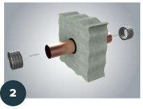
Install pipes or cables. Install backing material as required into annular space as shown to both sides of wall assembly.
