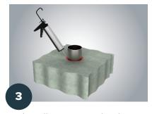
Apply caulking as required to close remaining gap to one side of floor assembly: providing a fire smoke and gas resistant seal. Spread caulking smoothly and evenly all around.
