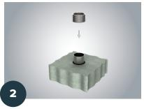
Install pipes or cables. Install backing material as required into annular space as shown on one side of floor assembly.
