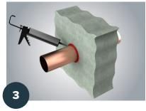
Apply caulking as required to close remaining gap to both sides of wall assembly; providing a fire smoke and gas resistant seal. Spread caulking smoothly and evenly all around.
